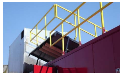
tilt roof and 2nd story hydraulically raised
